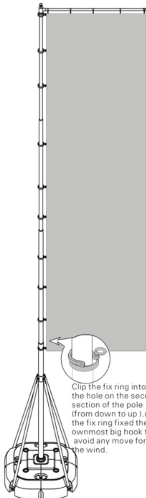
Clip the fix ring into the hole on the second section of the pole (from down to up ).use the fix ring fixed the downmost big hook to avoid any move for the wind.
